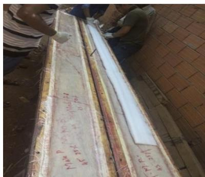
**Fig 10:** Filling airfoil mould with composite mixture
