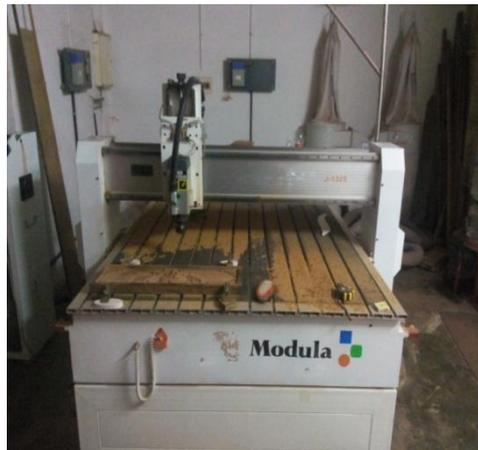
**Fig 2:** CNC router machine
