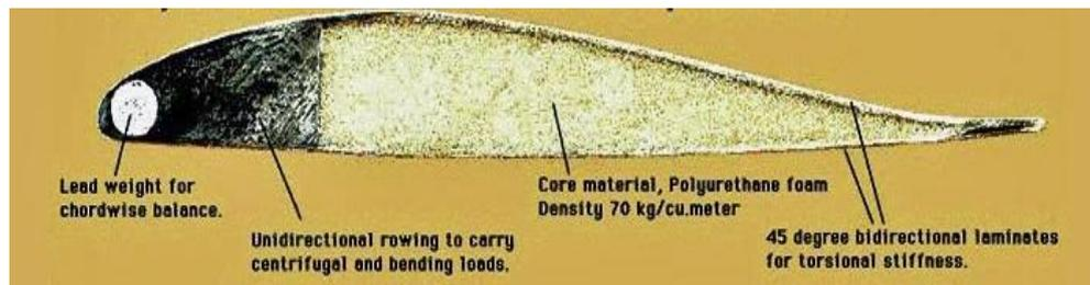
Fig 6: cross section of NACA 8-H-12 airfoil
